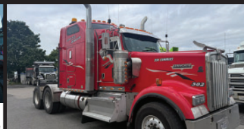
KENWORTH W900 2012 , Cummins ISX 550 hp, transm. Eaton RTLO18918B, ess. 14.6/46 lb, susp. Neway 52, 000 lb, ratio de différentiel 4.10 P.S.D. Tél.: 418-563-0340
