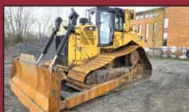
(2013) CATERPILLAR D6T LGP, 6S Tilt blade, drawbar (11,500 hrs.)
