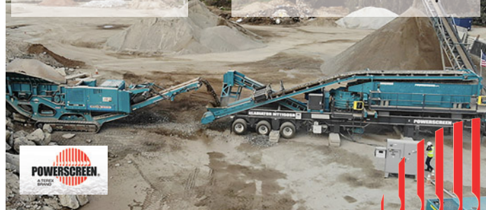
GLADIATOR MT1150SR Cône TC1150 & tamis 6x20 3 ponts
