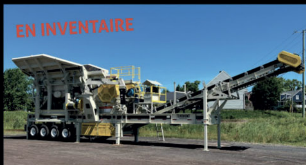
Station primaire Metso C-120 – Capacité 800 TPH
