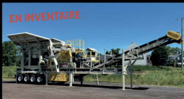
Station primaire Metso C-120 – Capacité 800 TPH
