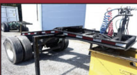
Fardier (2019) HC Jeep Dolly 1 essieu, 5 th wheel ajustable, budd wheel aluminium, air suspension
