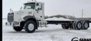
MACK GRANITE GR64B9 2020 374,500KM #C-37167 CUMMINS L9 350HP / ALLISON / 18 000 - 40 000 LBS
