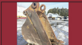
ATTACHMENT: Bucket 30" (4 dents) excavatrice 30 à 36 tonnes
