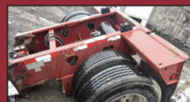
(2014) Fardier : TRAIL KING, essieu amovible /flip axle, suspension à air, budd wheels aluminium
