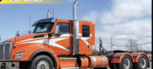
KENWORTH T880 2024 #C-37442 CUMMINS X-15E 565HP / 18 VIT. / 20 000 - 46 000 LBS
