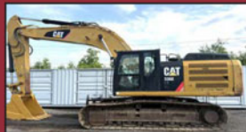
(2014) CATERPILLAR 336 ELH (Hybride electric) ,lock valves, aux. hydraulic piping, (9,300 hrs.)
