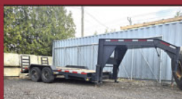
Remorque Goose neck (2013) CAM Superline 25' x 102", rampes arrières, essieux 12,000 lbs
