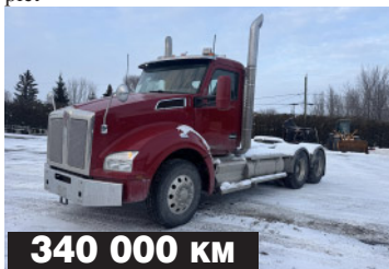
KENWORTH T880 2019 , Day Cab, Cummins ISX 500 hp, Ultra Shift 12, 14/46 "Full Lock", Wet line kit
