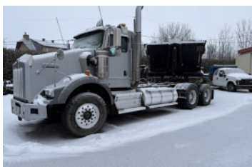
KENWORTH T800 2008 , 500 hp, cummins, 18 vitesses, 16/46 lb., susp. air, "Wet Kit"
