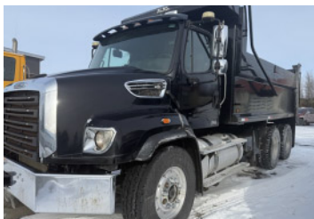
FREIGHTLINER SD114 2017 , DD13, 450 hp Allison, 16/46 lb., acns 15', attache arrière
