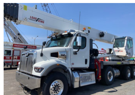
2025 LOAD-KING LK-40127S, flèche 31'/127', 5 sections, fléchette 30.5'/55'
