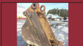
ATTACHMENT: Bucket 30" (4 dents) excavatrice 30 à 36 tonnes
